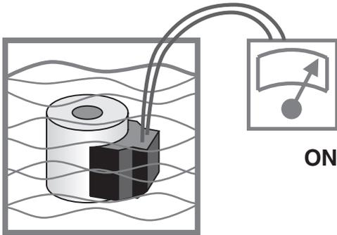
**In this test the coil is immersed while powered on.**
