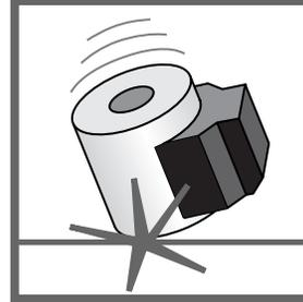
This test simulates the effects of dropping a coil while it is being handled.
