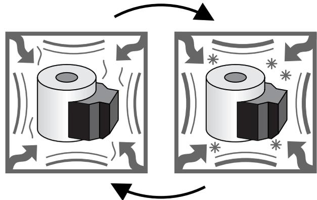
This test simulates the effects of storage in extreme temperatures for some time.
