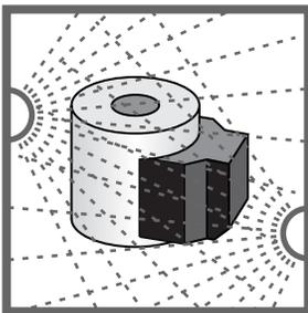
This accelerated test is designed to simulate the corrosive environment that the coil will encounter during the life of the vehicle.
