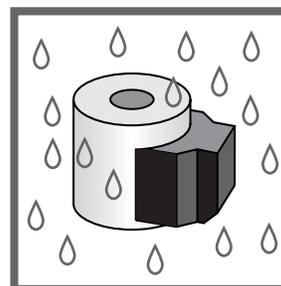
This test simulates the effects of relative humidity on the coil.
