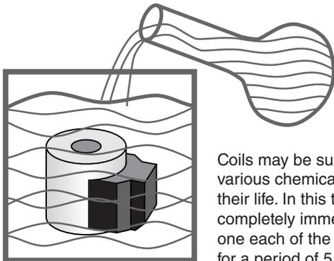
Coils may be subjected to various chemicals throughout their life. In this test a coil is completely immersed in only one each of the following fluids for a period of 5 minutes. Twelve coils are used at a time. After immersion the coils are heated
