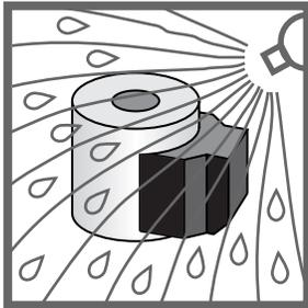
This test simulates high-pressure steam-jet cleaning of a component.
