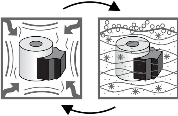
The purpose of this test is to try to induce cracks in the encapsulation of the coil.
