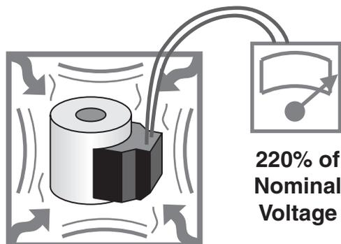
**This test simulates the voltage required to jump start heavy equipment.**
